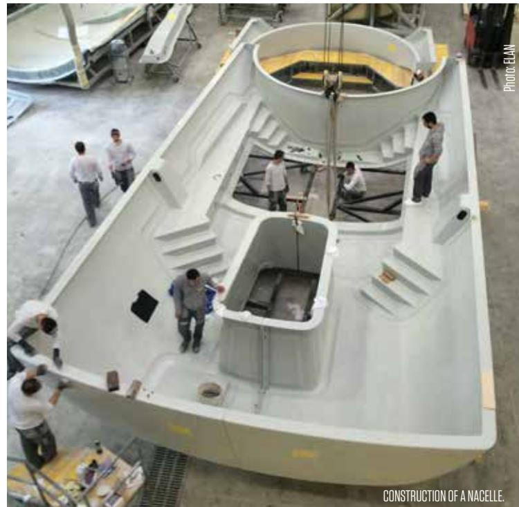
CONSTRUCTION OF A NACELLE.
